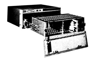
The EAI 380 Computing System is a completely new solid state 10 Volt desk-top computer with a capacity of 36 amplifiers. It is an advanced analogue/hybrid computer that is easy to understand and operate. For a minimum outlay you can obtain a 380 then expand with plug-in analogue and logic units at any time.
