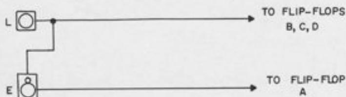
Figure 15.2. Internal Connections for the "Load" and "Enable" Inputs
