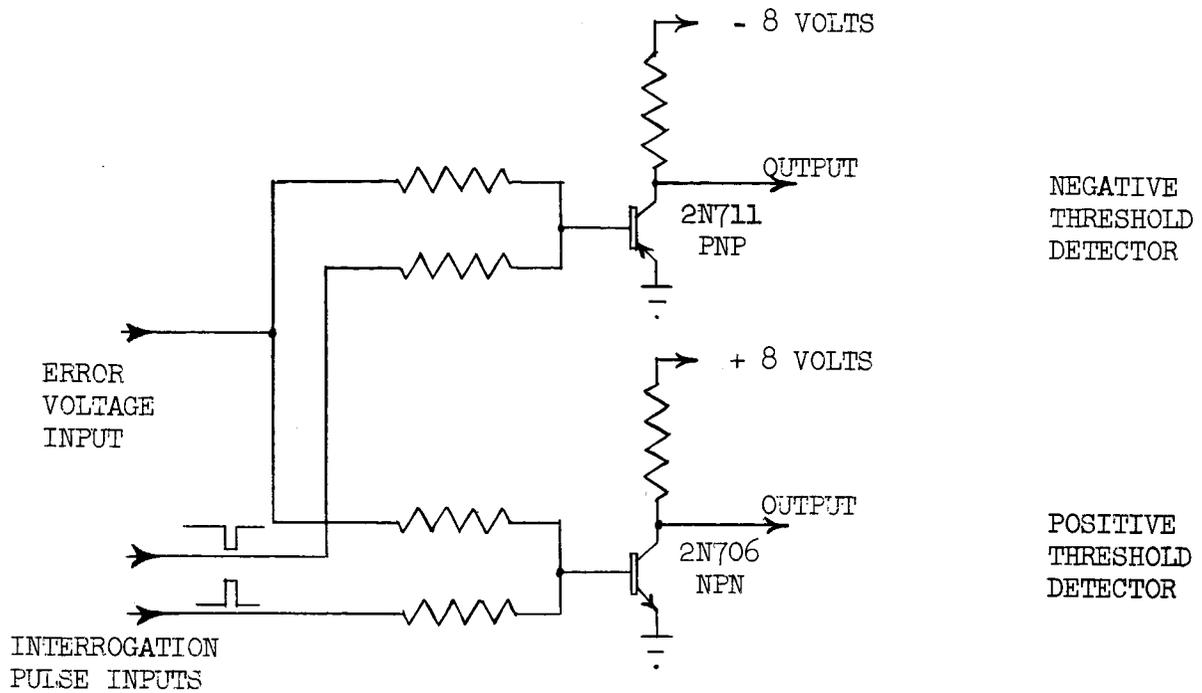
Figure 6: Circuit Diagram of the Threshold Detectors
