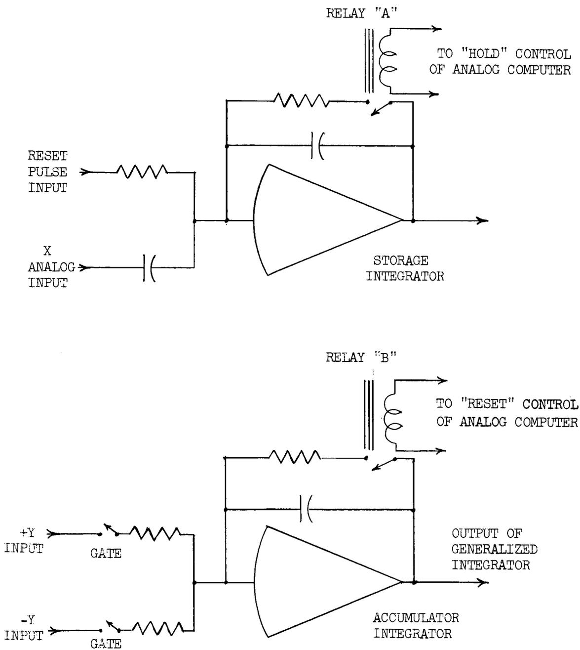
Figure 8: Analog Program of the Electronic Generalized Integrator
