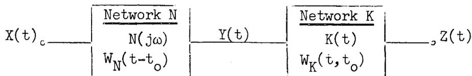
The behavior of the network N is well known; further, it is easy to show that since  $Z(t) = K(t)Y(t)$ , then  $E[Z(t)] = K(t)E[Y(t)]$  and the covariance function for  $Z(t)$  is given by
