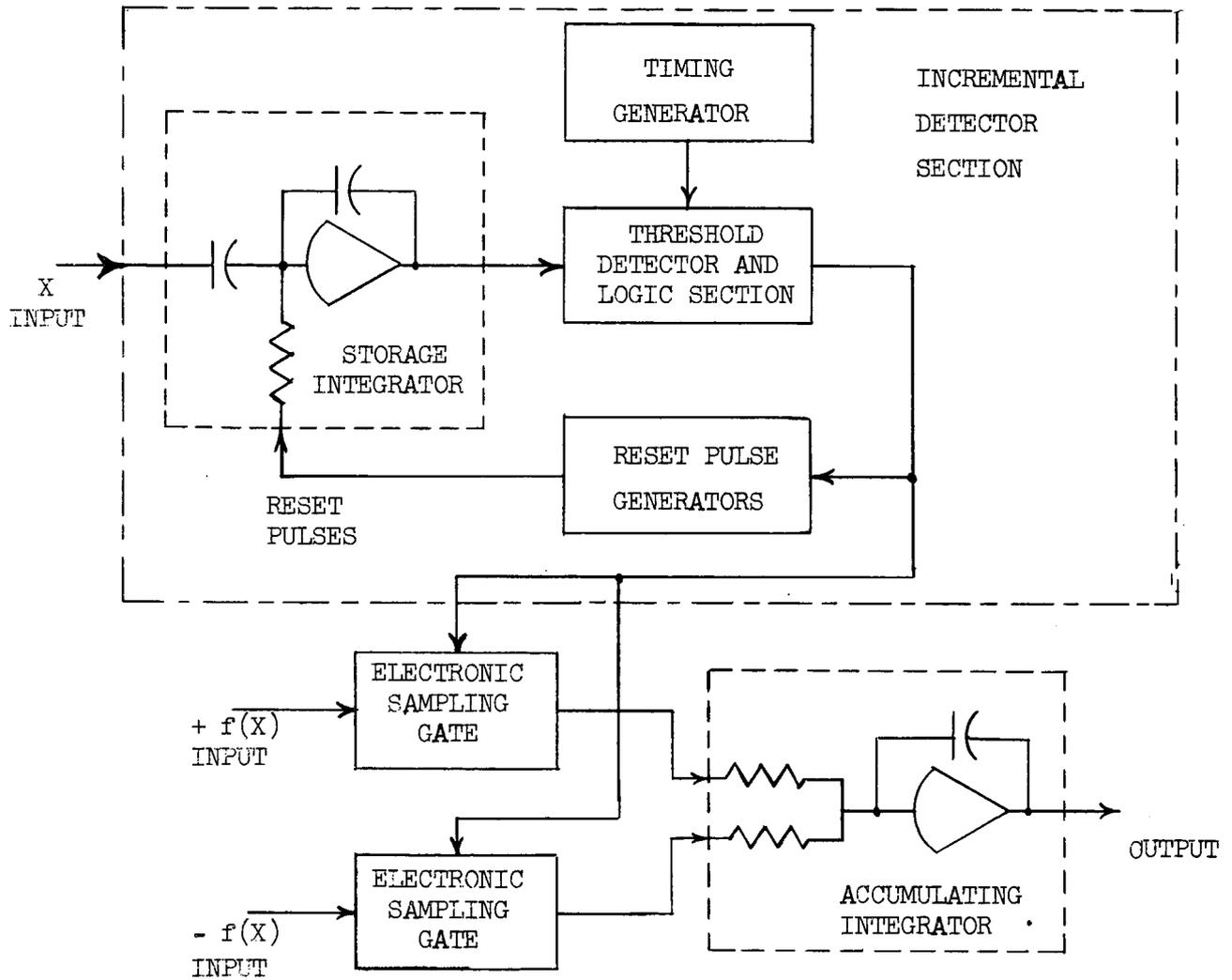
Figure 3: Basic Block Diagram of the Electronic Generalized Integrator
