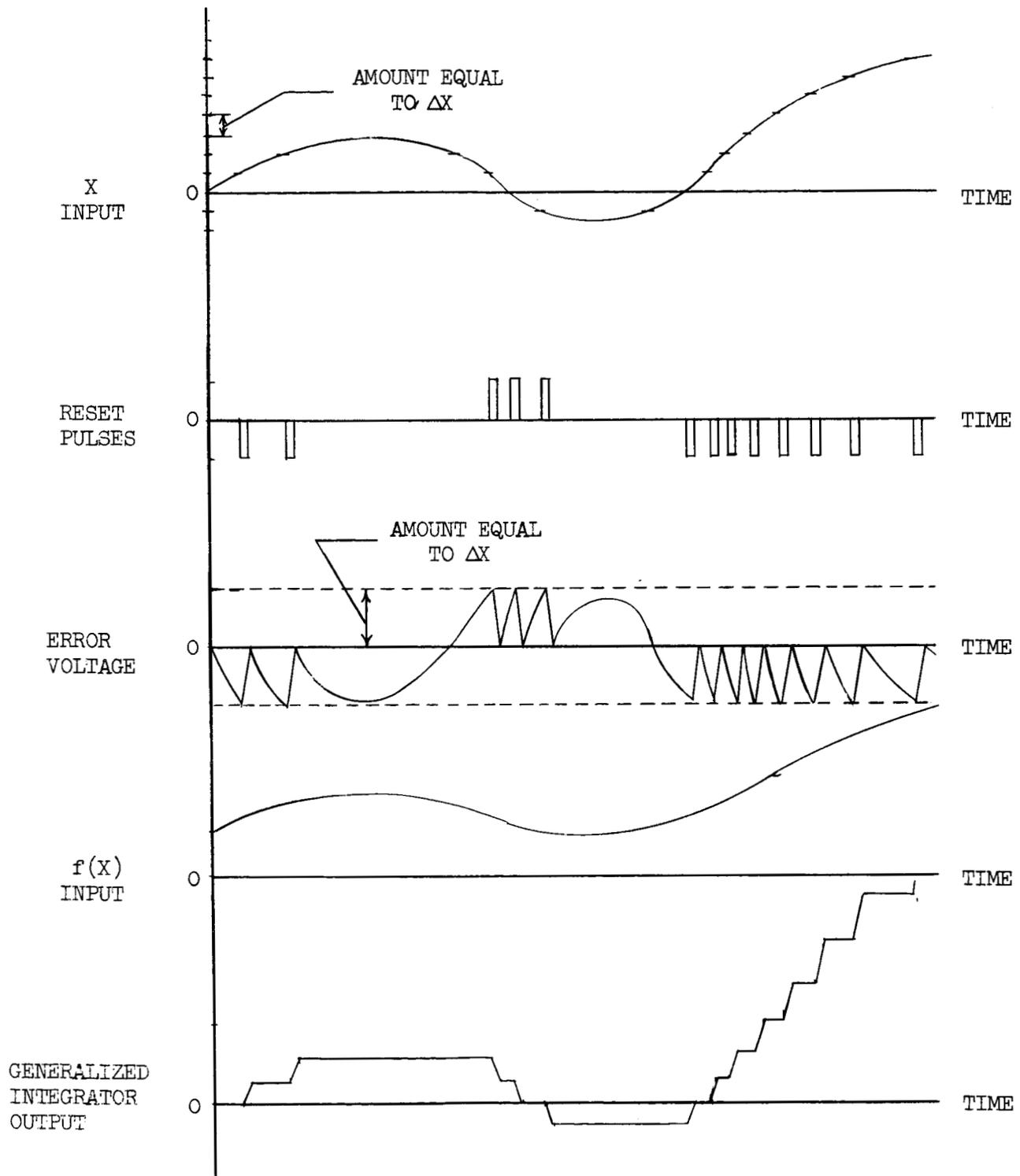
Figure 4: Typical Waveforms Found in the Electronic Generalized Integrator
