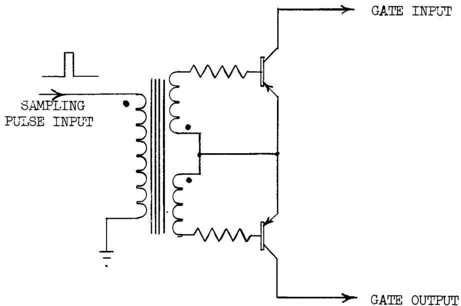
Figure 7: Circuit Diagram of the Electronic Sampling Gates
