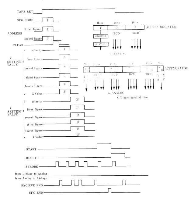
Note: On the setting procedure for a function generator a program of the digital computer must be prepared in order that the setting is proceeded from the maximum negative value toward the maximum positive value of X axis.
