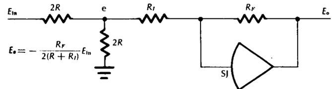
Figure 6 — Binary-weighted digital attenuator
