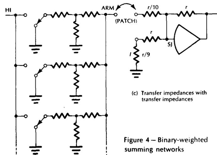
Figure 4—Binary-weighted summing networks
