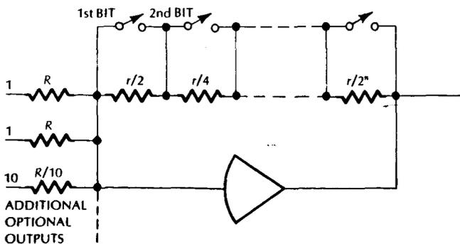
Figure 7 — Simple version of a summing amplifier with switched gain
