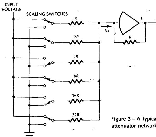
Figure 3—A typical attenuator network
