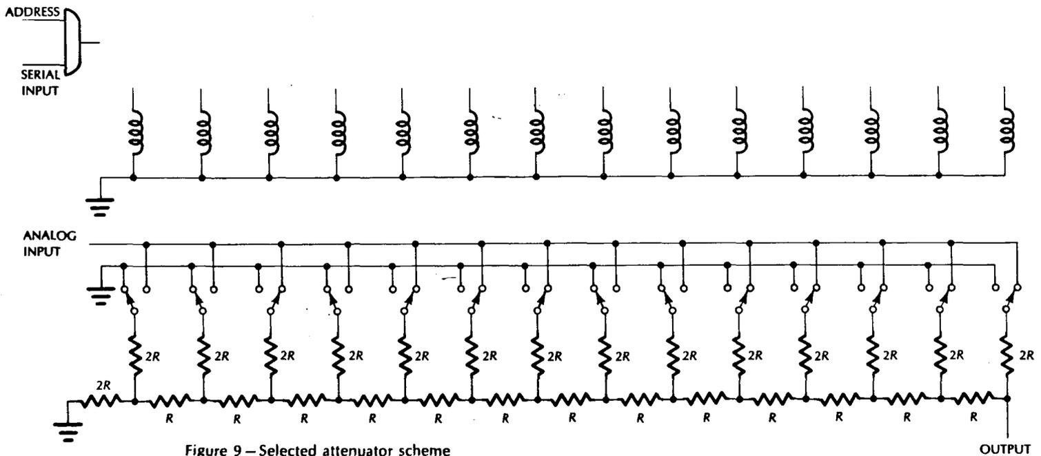
Figure 9—Selected attenuator scheme
