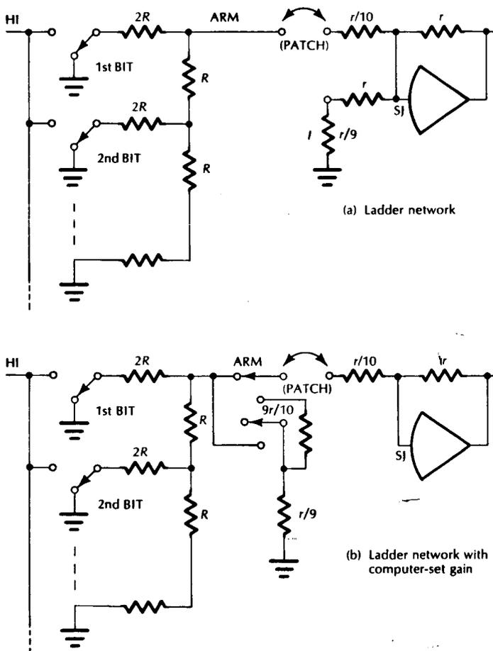
Figure 5 — Binary-weighted-ladder summing networks
