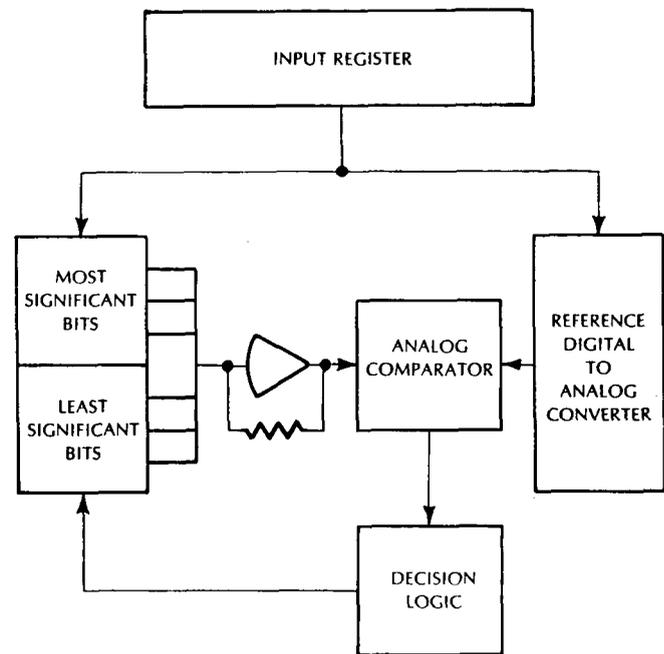
Figure 8 — Simplified block diagram of a digital attenuator employing error feedback
