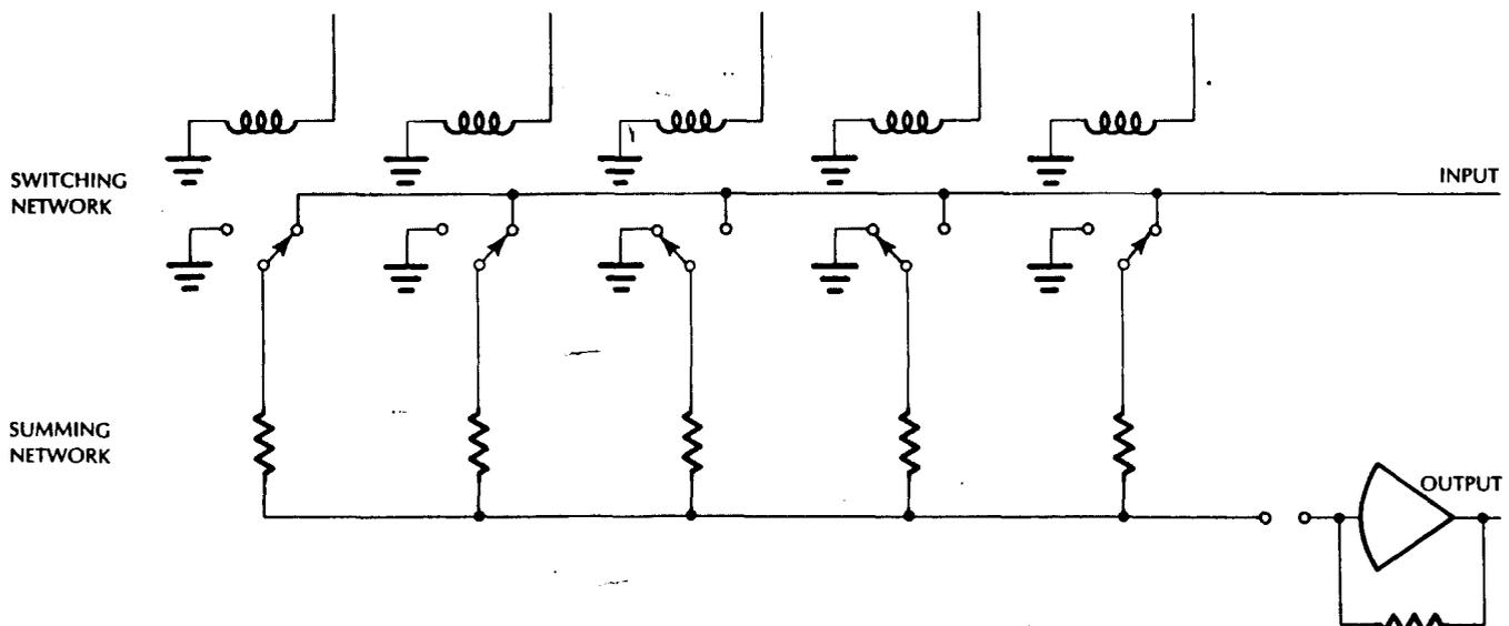
Figure 2 — A typical digital-attenuator
