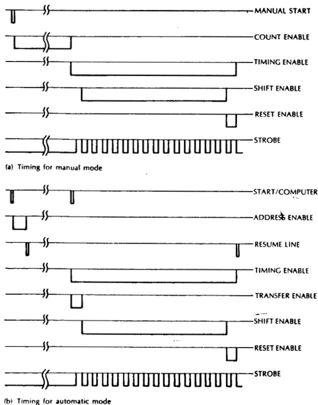
Figure 13 - Timing diagrams
