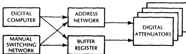
Figure 1 - A digital attenuator system
